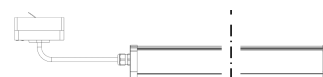
Connection cable from the luminaire end cap 3x1.5mm 2 with universal 3-phase adapter
